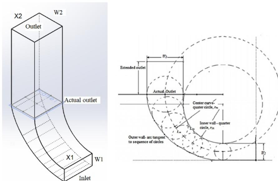
Fig. 1 - 90° curve diffuser model
