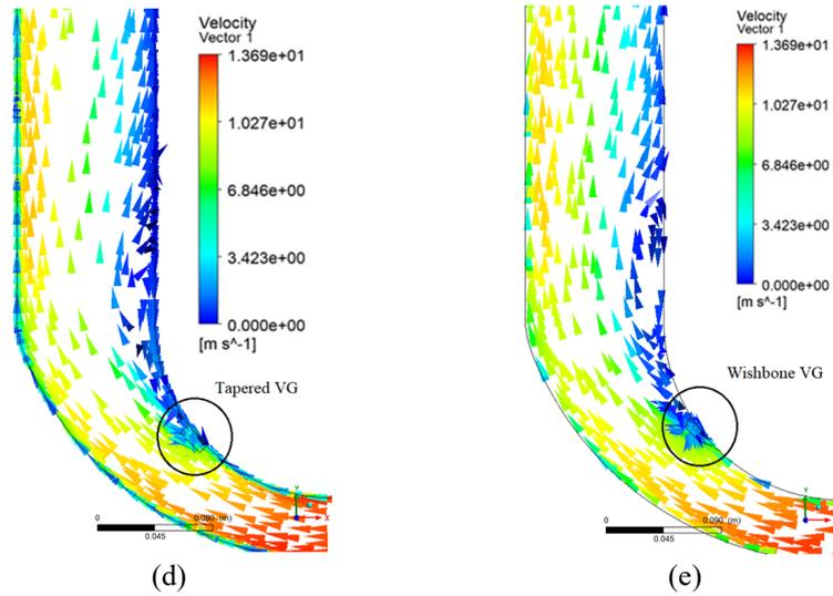
Fig. 5 - Flow characteristics of curve diffuser (a) without VG; (b) with rectangle VG; (c) with triangle VG; (d) with tapered VG; (e) with wishbone VG
