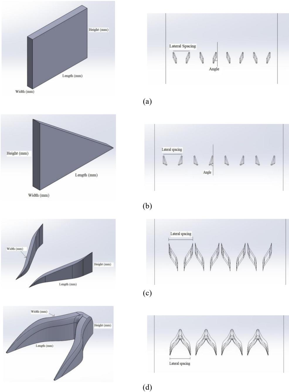
**Fig. 2 - Types and configurations of vortex generator (a) rectangle; (b) triangle; (c) tapered; (d) wishbone**
