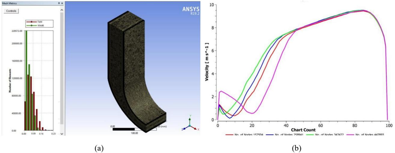
Fig. 3 - (a) hybrid mesh with enhanced wall treatment of  $y^+ \approx 1.0$ ; (b) grid independence test result
