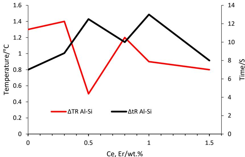
**Fig. 4 - Effect of Ce, Er concentration on recalescence temperature  $\Delta T_R^{Al-Si}$  and time  $\Delta t_R^{Al-Si}$**
