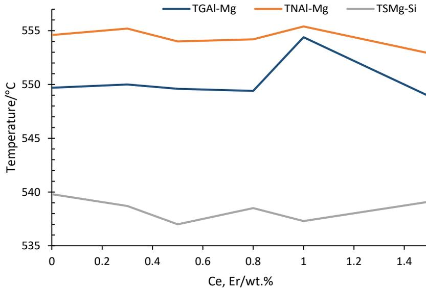
**Fig. 5 - Variation of TGAl-Mg, TNAl-Mg for base alloy and different concentrations of Ce, Er addition and end of solidification temperature TSMg-Si of base alloy and different Ce levels in the alloy**
