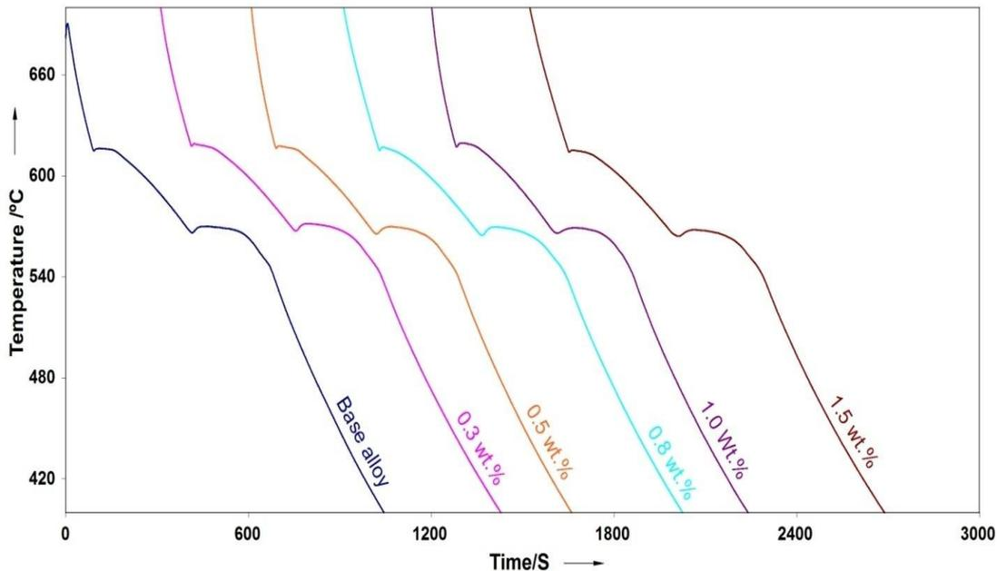
Fig. 1 - Cooling curve of base alloy and alloys treated with additions Ce and Er treated alloys
