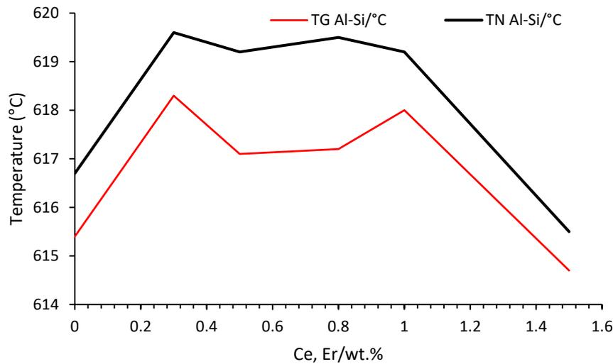
**Fig. 2 - Changes of hypoeutectic growth temperature TG Al-Phase, and nucleation temperature TN Al-Phase with different concentration of Ce, Er**
