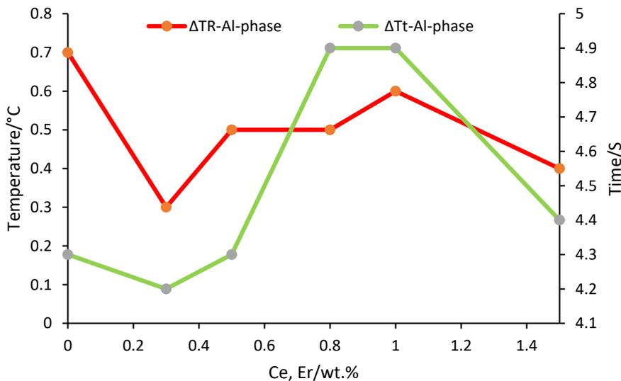
**Fig. 3 - Effect of Ce, Er concentration on recalescence temperature ΔTR Al-Phase and time ΔtR Al-Phase**
