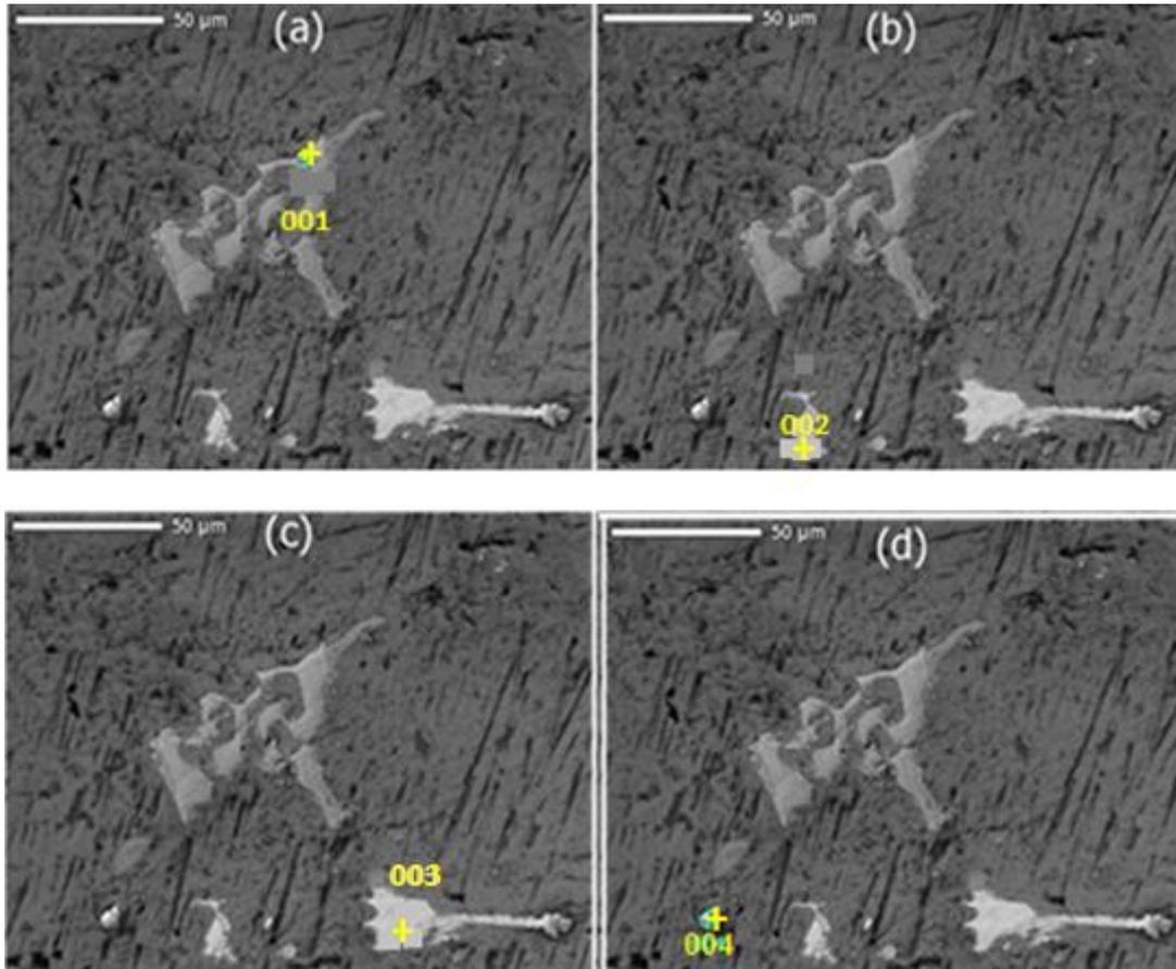
Fig. 8 - SEM/EDS micrograph of the specimen without and with 1.5 wt.% Ce, Er (a) Al-Si-Fe-Er; (b) Al-Si-Ce-Er; (c) Al-Si-Ce-Er; (d) Al-Si
