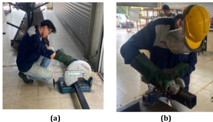
Fig. 2 Cutting of the mild steel components using (a) Cut off machine; (b) Hand grinder
