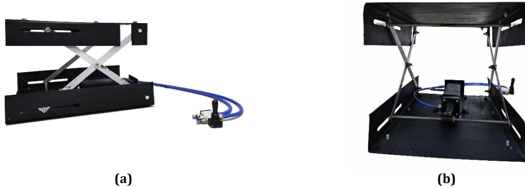
Fig. 4 The fully assembled pneumatic scissor lifting jack integrated with a directional control valve, from (a) Side view; and (b) Front view
