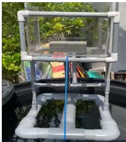
Fig. 6 Baby-cot prototype under a 3.0 kg payload during the 30-minute floatation test
