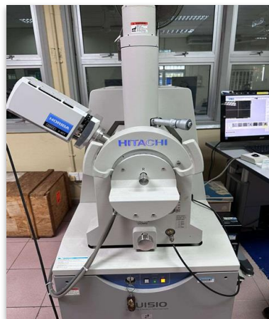
Fig. 6 Scanning electron microscope (SEM; Hitachi SU1510)
