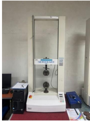
Fig. 3 Universal testing machine (AGS-5KN, Japan)
