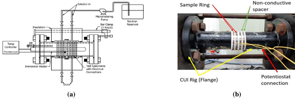
**Fig. 1 - (a) Schematic layout of CUI simulation equipment [10]; (b) sample ring and spacer position**
