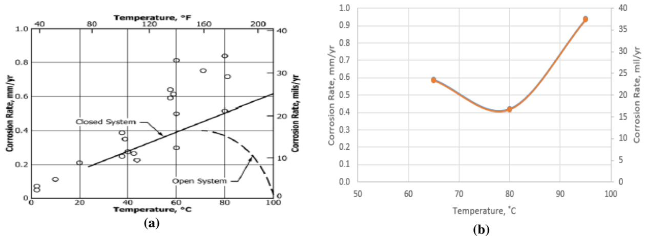
**Fig. 4 - (a) Comparison of actual plan CUI corrosion rates measurements (Open Data Points Shown is for Plant CUI) with Laboratory Corrosion data obtained in open and closed systems [11]; (b) CUI corrosion rates obtained using laboratory simulation**
