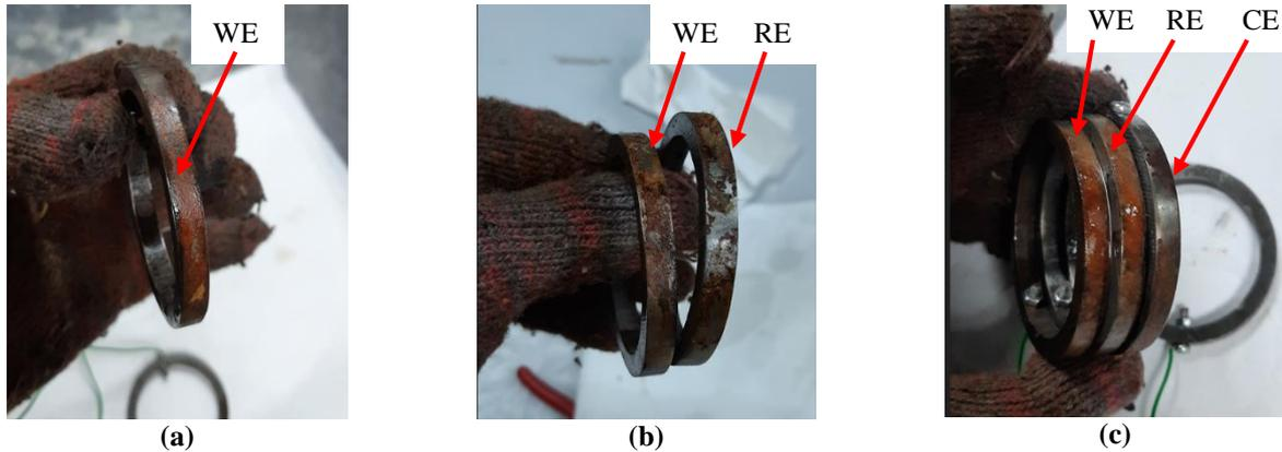
**Fig. 2 - Sample ring condition after being exposed under insulation at (a) 65°C; (b) 80°C and; (c) 95°C**
