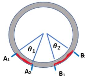
**Fig. 3 - Marking the corroded surface area**
