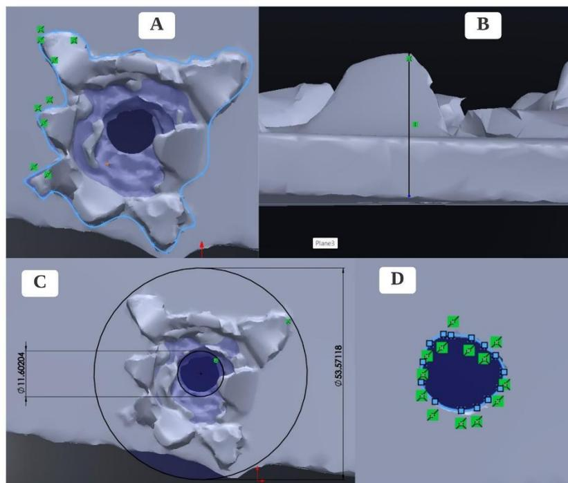
**Fig. 3 - 3D scan deformation profile capture (a) deformation profile of the exit wound; (b) maximum depth of the crater; (c) bullet hole diameter and; deformation zone; (d) deformation profile of the entry wound**
