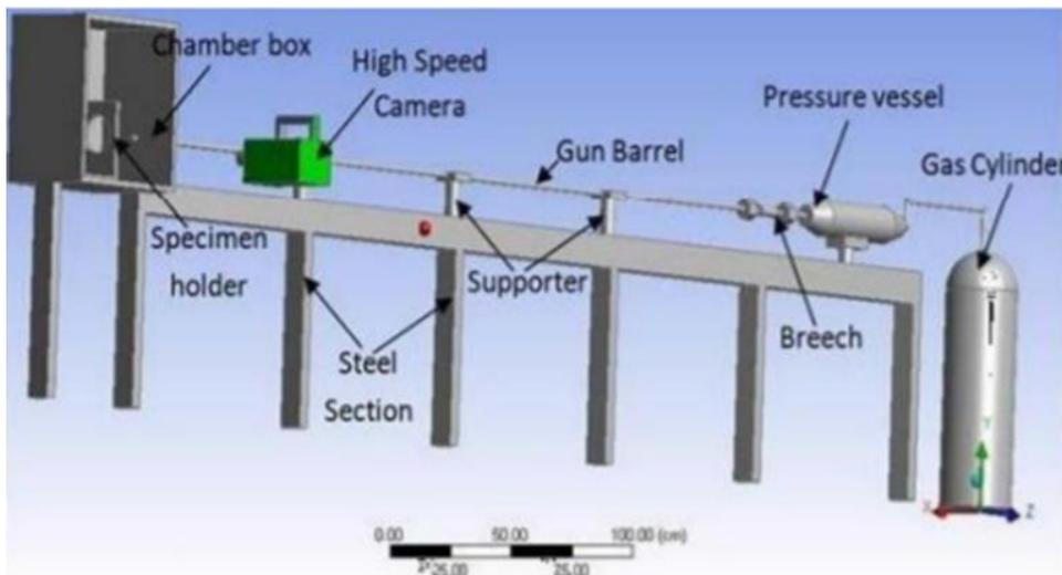
Fig. 1 - Single stage gas gun setup [16]
