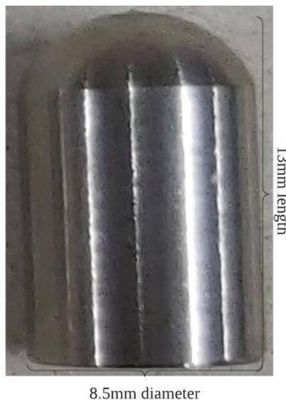
Fig. 2 - Hemispherical impactor used in tests
