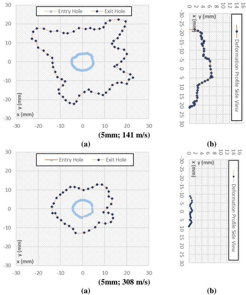
Fig. 5 - Deformation profile of recycled AA 6061 plates (a) bullet entry and exit hole profiles; (b) side view of the deformation
