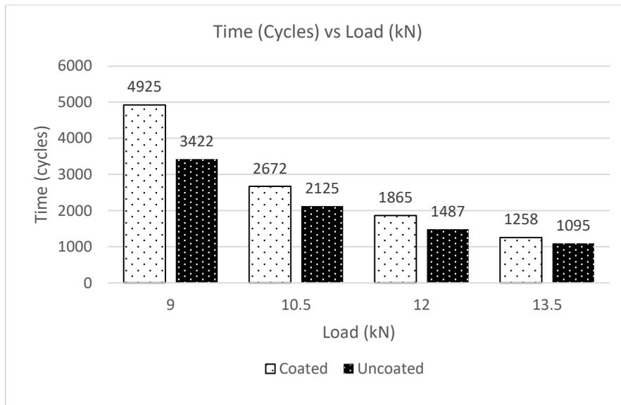
**Fig. 3 - Bar chart of fatigue life for all forces for uncoated and coated specimens**
