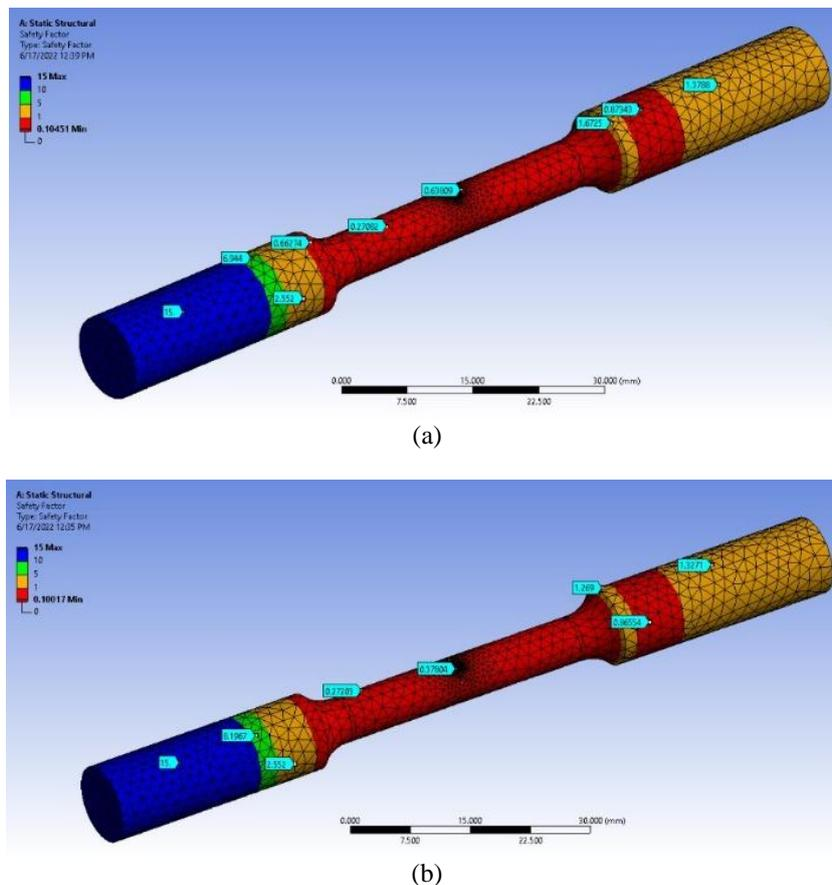
**Fig. 6 - Result of fatigue safety factor for (a) the uncoated specimen and; (b) the coated specimen**
