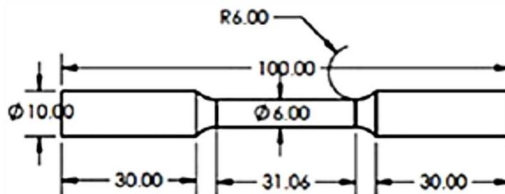
**Fig. 1 - Dimension of the specimen**
