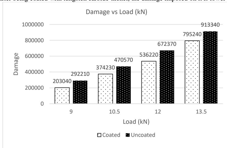
**Fig. 4 - Bar chart of fatigue damage for all forces for uncoated and coated specimens**
