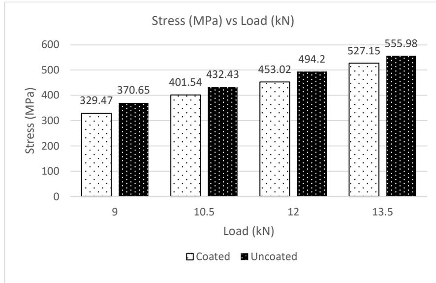
**Fig. 5 - Bar chart of fatigue strength for all forces for uncoated and coated specimens**
