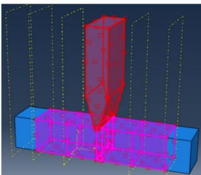
Fig. 3 - The specimen model's and striker model's surface-to-surface contact
