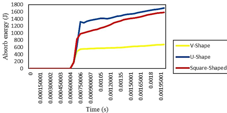
**Fig. 8 - Absorb energy versus time graph of aluminium alloy 6061 with various side groove shapes**
