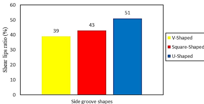
Fig. 6 - Relationship of side groove shapes toward the shear lips formation ratio
