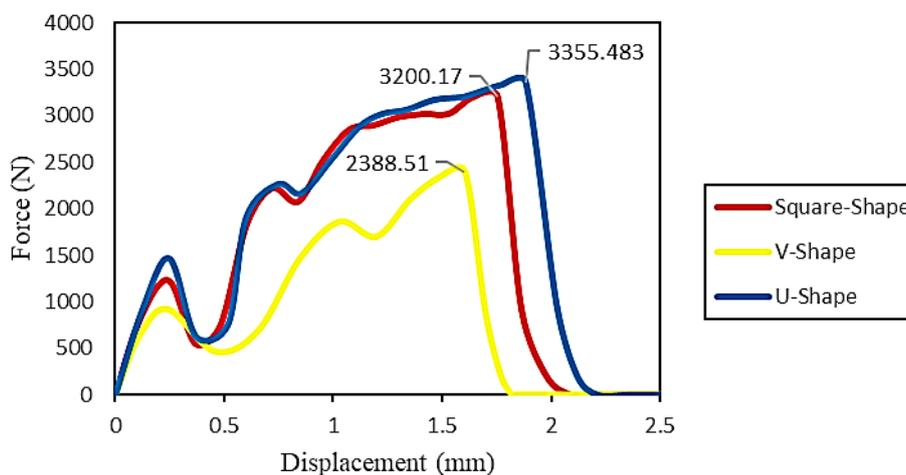
Fig. 10 - The force versus displacement graph for each of the side groove forms
