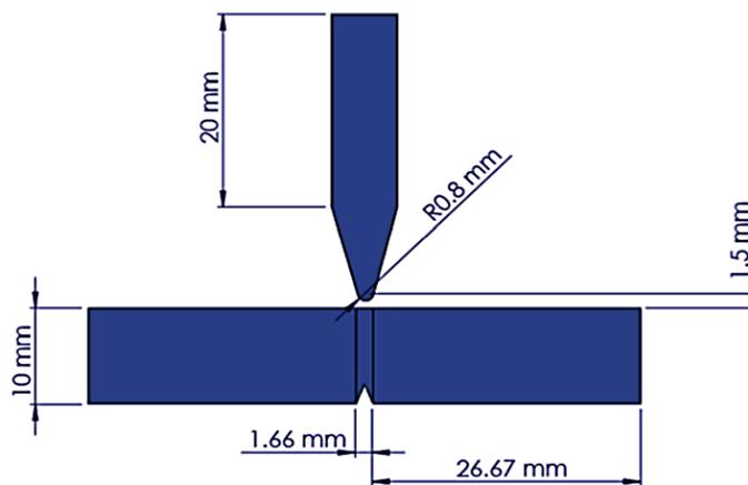
Fig. 1 - The Charpy impact test full assembly with their dimensions
