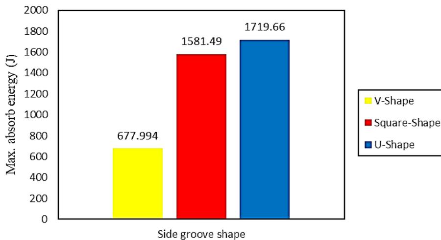
**Fig. 7 - The bar chart represents the maximum energy absorbed against the different types of side groove shapes**
