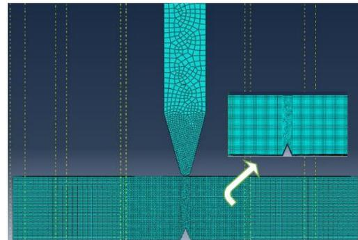
Fig. 4 - The Charpy impact test model has fully meshed
