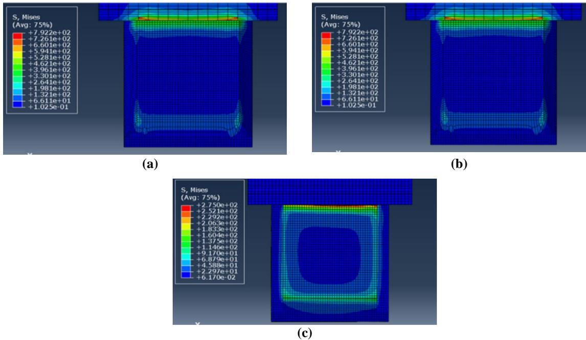
Fig. 5 - Specimen surface that contains the formation of the shear lip for various shape grooves, (a) V-shaped; (b) Square-shape; (c) U-shaped
