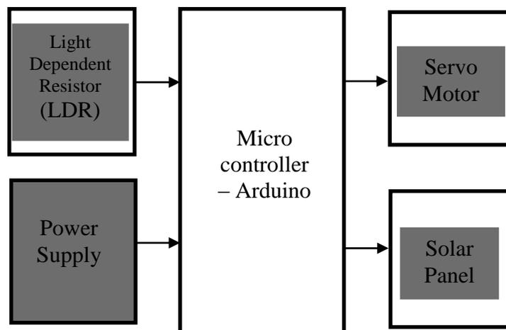
Fig. 2 - Solar Tracking System block diagram
