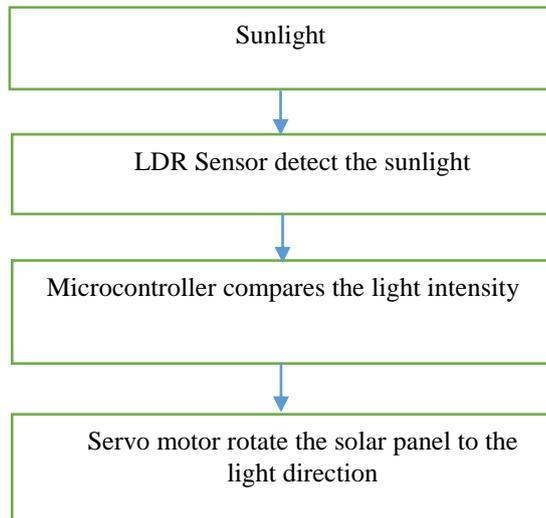
Fig. 1 - Solar Tracking System flowchart
