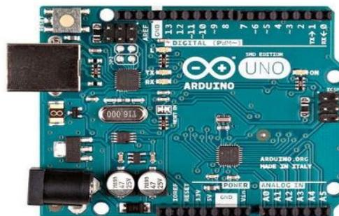
Fig. 3 - Arduino Uno microcontroller
