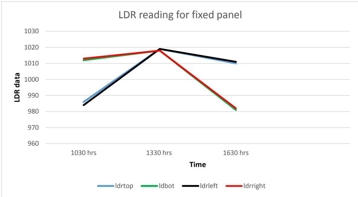
**Fig. 8 - Result for Fixed Solar Panel**
