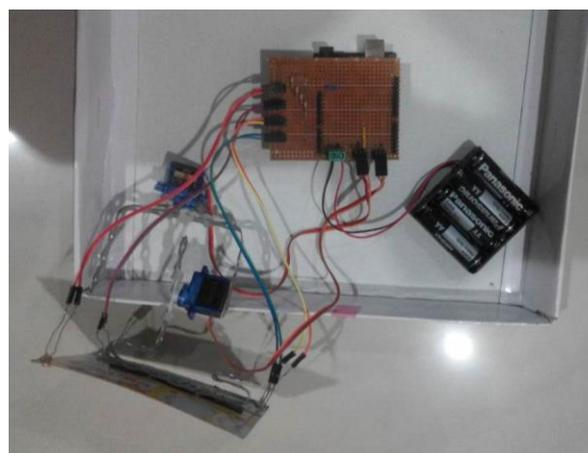
**Fig. 6 - Complete circuit of Solar Tracking System**
