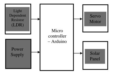
Fig. 2 - Solar Tracking System block diagram
