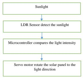
Fig. 1 - Solar Tracking System flowchart
