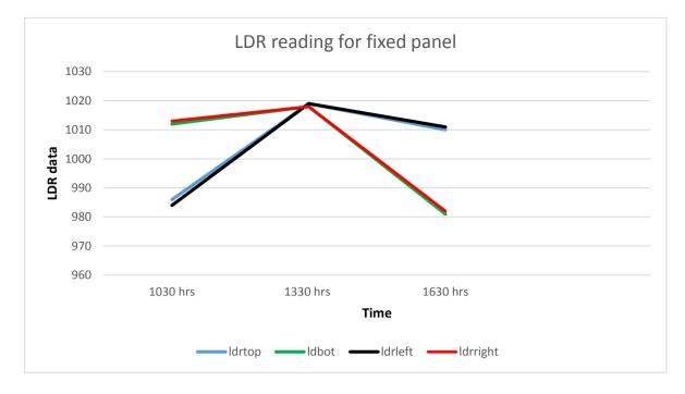
Fig. 8 - Result for Fixed Solar Panel
