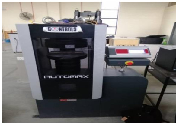
Fig. 4 - Compression Testing Machine
