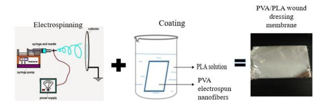
Fig. 2 - Preparation of polyvinyl alcohol nanofiber mat coated with poly(lactic acid)
