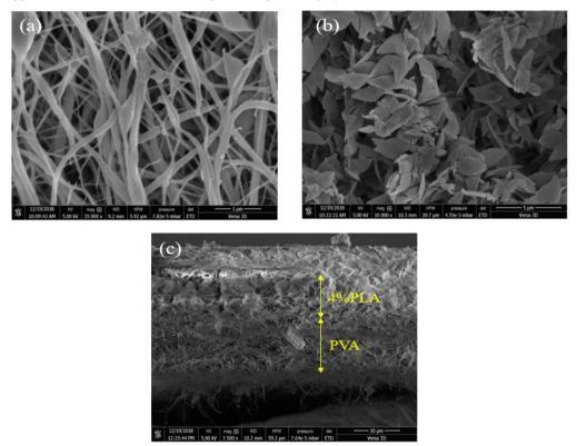
Fig. 4 - FE-SEM image of (a) neat PVA nanofiber, (b) PVA nanofiber coated with 4% PLA and (c) cross-section of PVA nanofiber coated with 4% PLA
