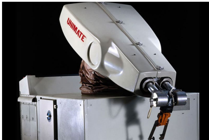
Fig. 1 Unimate- the first industrial robot
