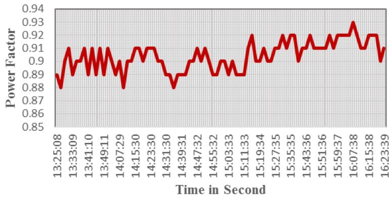
**Fig. 8** Measured power factor of the tested residential building
