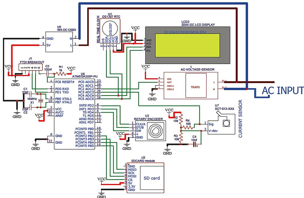
Fig. 2 Circuit diagram of the smart energy meter
