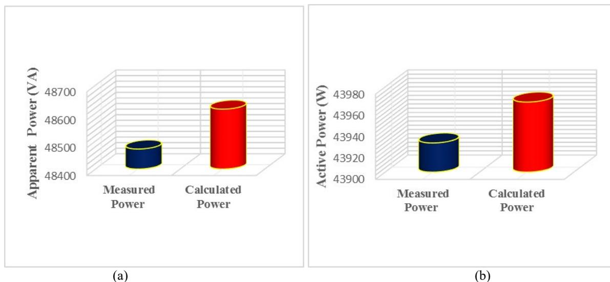
**Fig. 8** Graph measured power and calculated power of (a) Apparent power; (b) Active power
