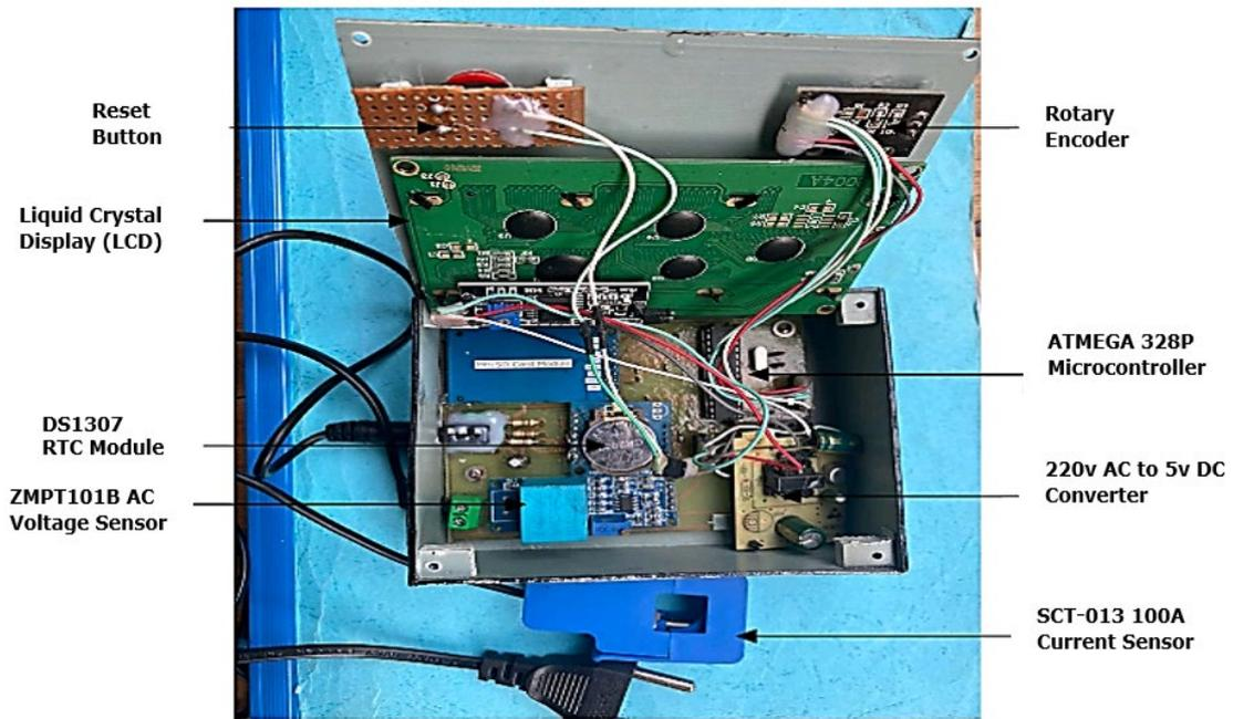
**Fig. 3** Development of smart energy meter
