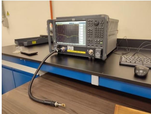
Fig. 8 - The measurement of proposed antenna using VNA
