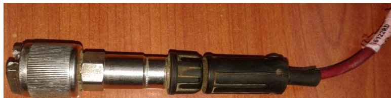
Fig. 2 - Accelerometer probe with magnetic base for onsite data capture
