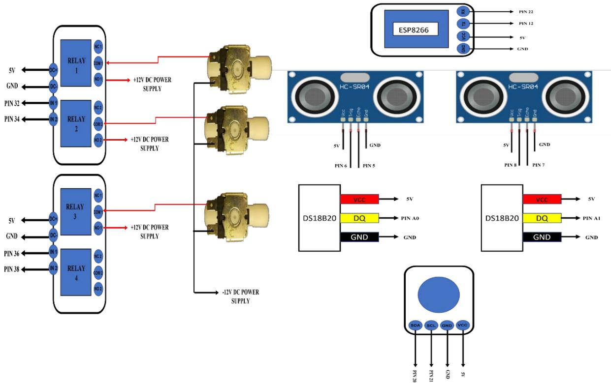
**Fig. 5 - Components connection to Arduino Mega 2560 Pinout**
