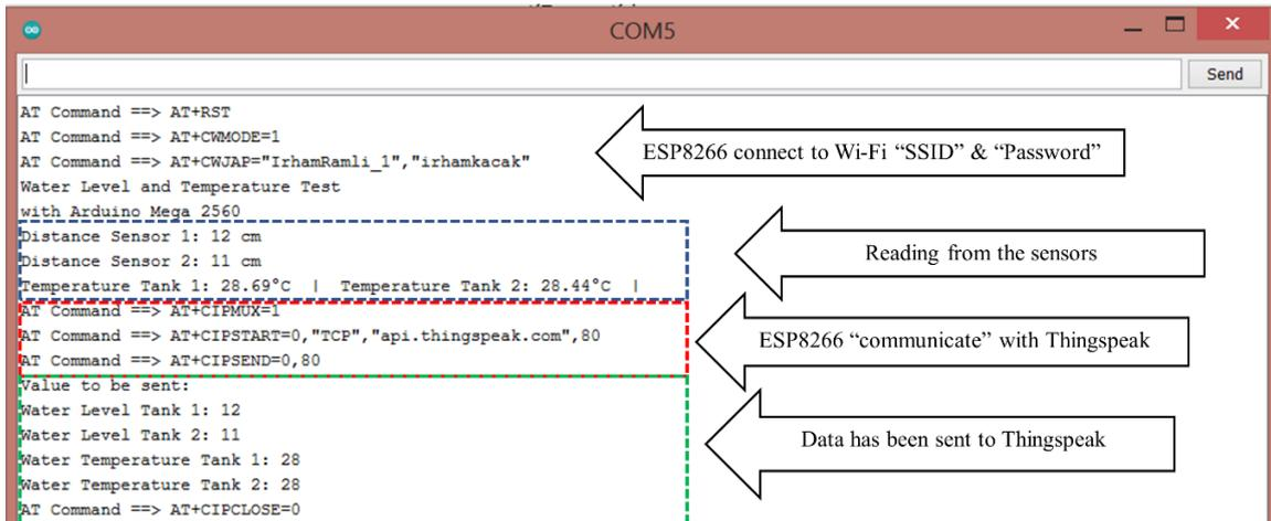
**Fig. 7 - Serial monitor display for monitoring system**
