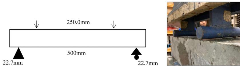
Fig. 4 - Four-Point Flexural Test Setup
