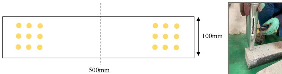
Fig. 3 - Test point of Rebound Hammer on the surface of the specimen
