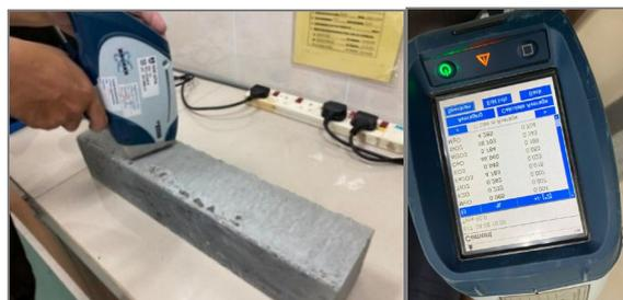
**Fig. 2 - Portable XRF used to detect the element composition of the concrete surface**
