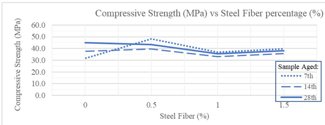
**Fig. 6 - The compressive strength (Mpa) vs steel fiber percentage (%)**
