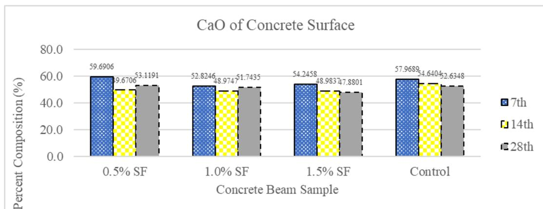
Fig. 5 - Composition of Calcium Oxide, CaO for concrete surface
