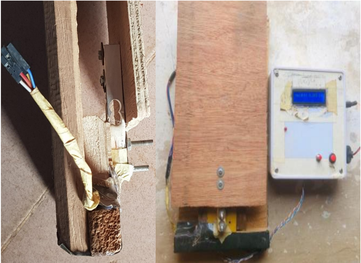
Fig. 5 - The Load Cell with Support Structure
