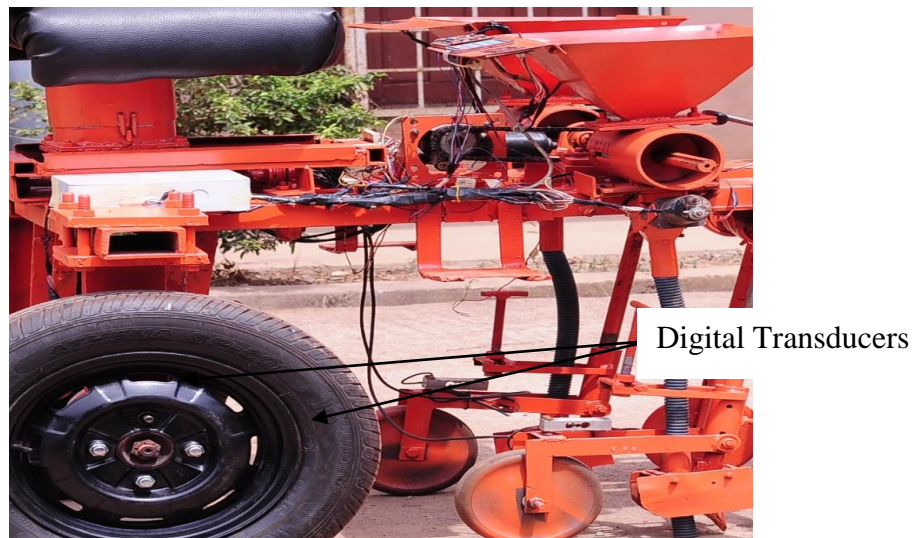
Fig. 7 - Transducer Attachment to the Press Wheels
