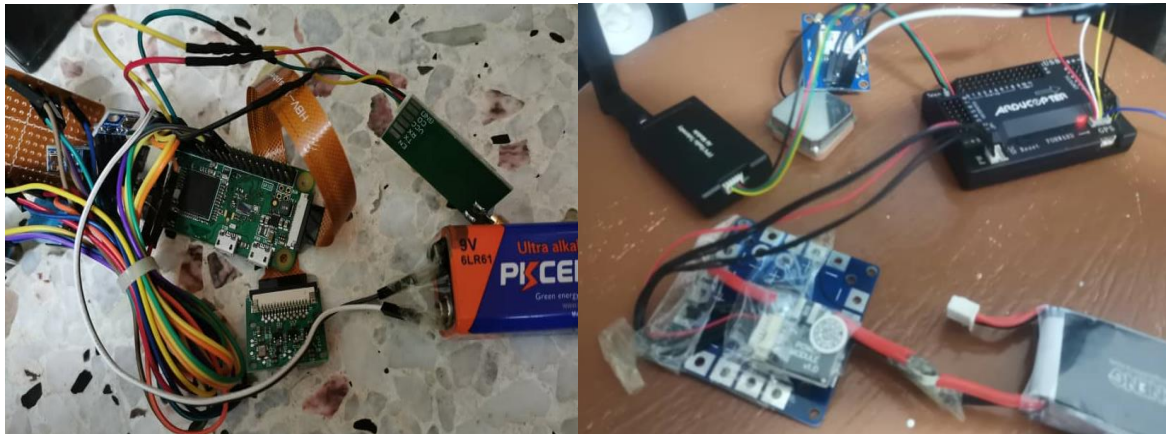
Fig. 6 - Power system integrate to Raspberry Pi and APM 2.8
