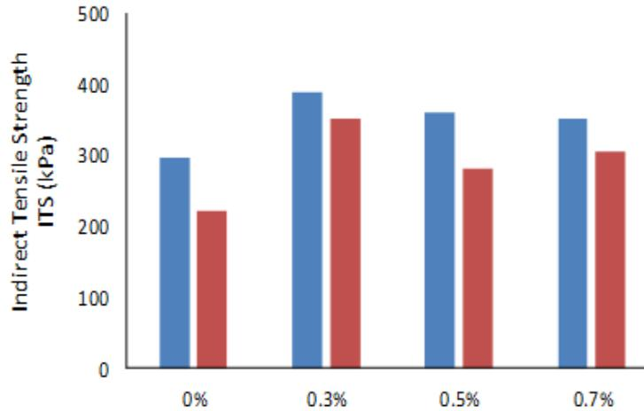
**Fig. 8 - Indirect Tensile Strength (ITS) with different steel fiber content**
