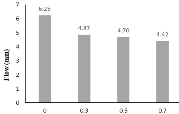
Fig. 6 - Flow values with different steel fiber content
