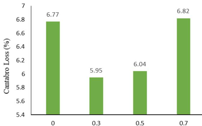
Fig. 7 - Cantabro loss values with different steel fiber content
