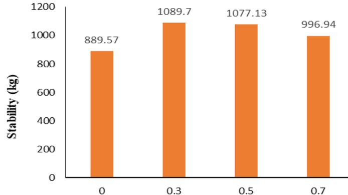
**Fig. 5 - Stability values with different steel fibre content**
