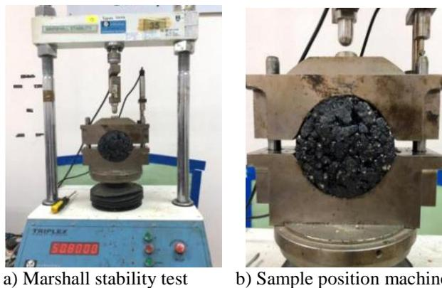
Fig. 2 - Marshall stability test
