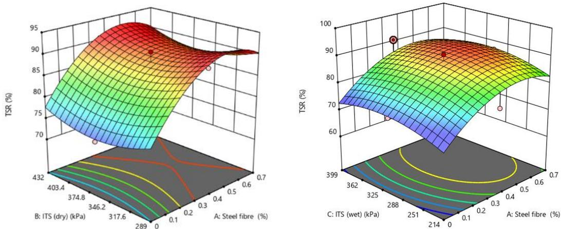
**Fig. 12 - Response surface model for tensile strength ratio**
