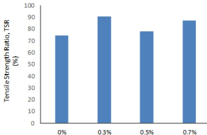
**Fig. 9 - Tensile Strength Ratio (TSR) with different steel fiber content**
