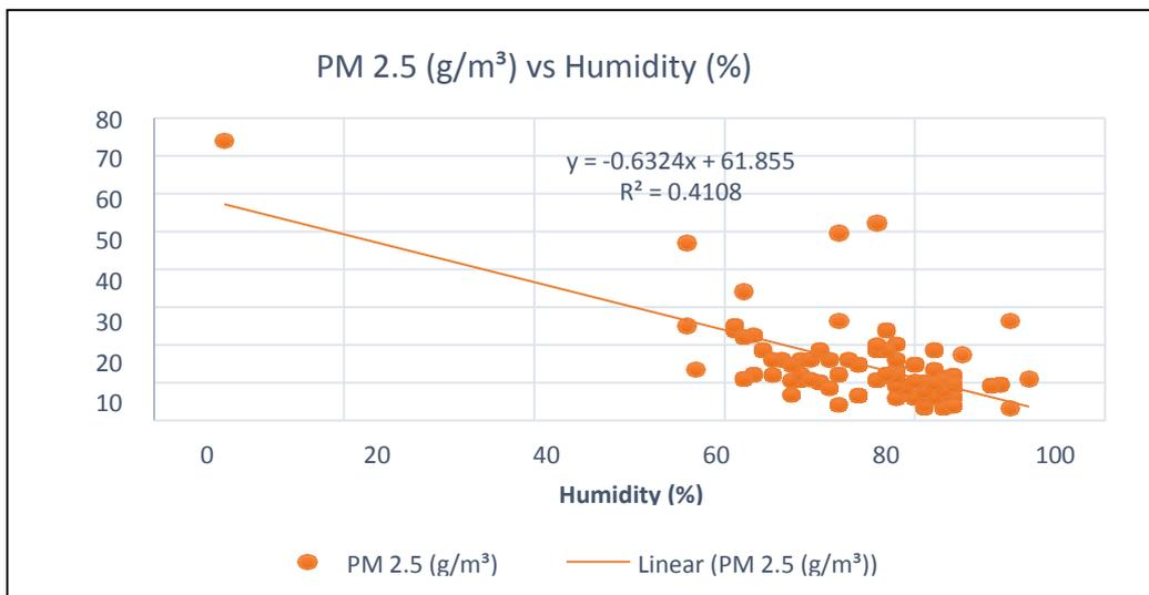
**Fig. 4 - Graph of correlation between PM<sub>2.5</sub> and humidity (%) for phase 2 at Station B**
