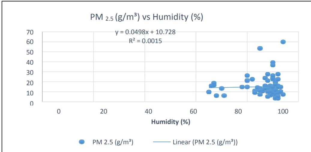
**Fig. 3 - Correlation graph between PM<sub>2.5</sub> and humidity (%) for phase 1 at Station B**
