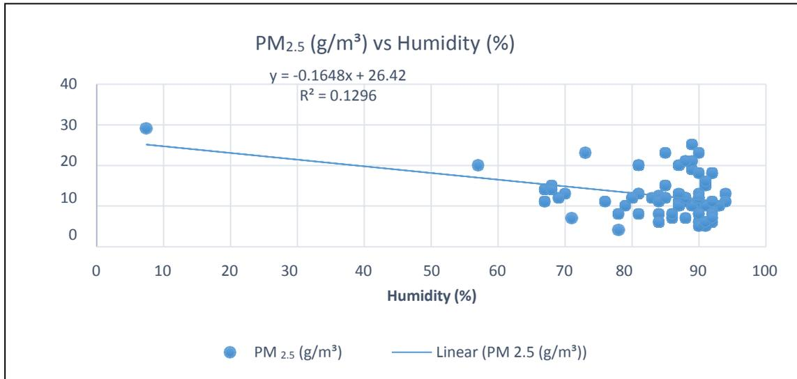
**Fig. 1 - Graph of correlation between PM<sub>2.5</sub> and humidity (%) for phase 1 at Station A**
