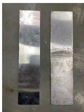
Fig. 1 Aluminium electrode used for the electrocoagulation process
