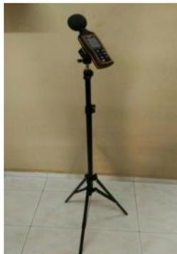
**Fig. 3 - Sound level meter on the tripod stand**
