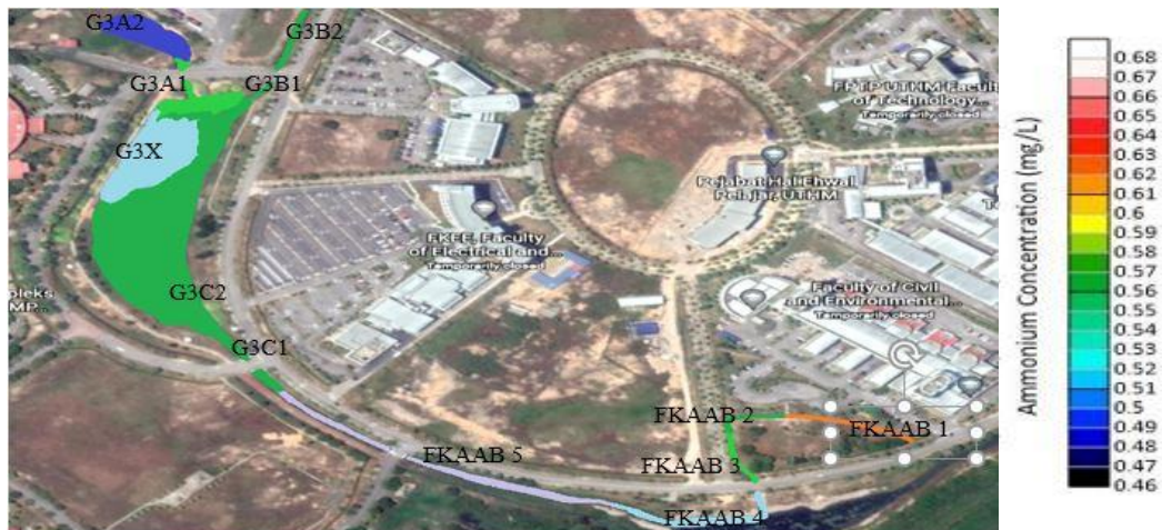
Fig. 5 - Ammonium concentration map along the Faculty of Civil Engineering and Built Environment and G3 Lake in week 3
