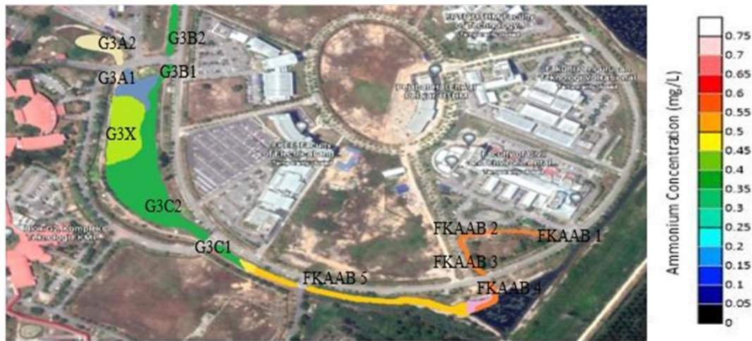
Fig. 3 - Ammonium concentration map along the Faculty of Civil Engineering and Built Environment and G3 Lake in week 1
