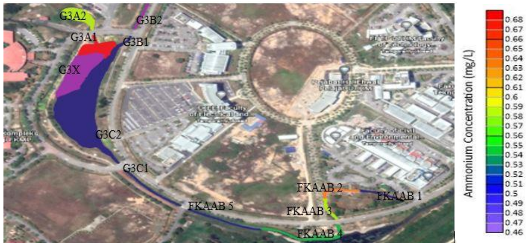
Fig. 4 - Ammonium concentration map along the Faculty of Civil Engineering and Built Environment and G3 Lake in week 2
