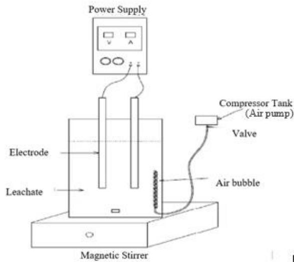
Fig. 2 - Aerated electrocoagulation process
