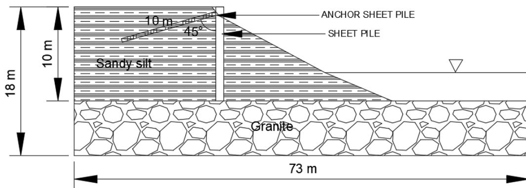
Fig. 1 Modelling of anchor sheet pile
