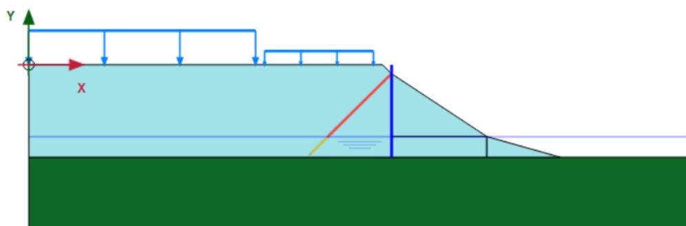
Fig. 2 Modelling of anchor sheet pile by using Plaxis 2D
