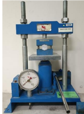
Fig. 4 Brazilian test equipment
