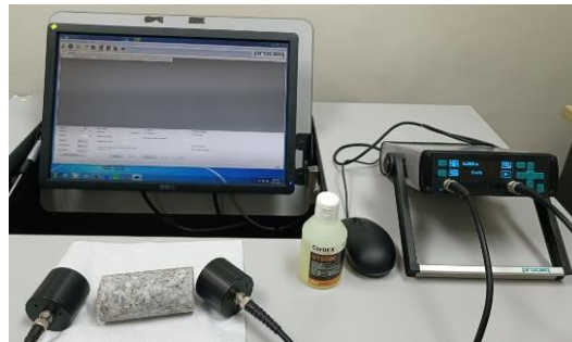
Fig. 2 The arrangement of PUNDIT test
