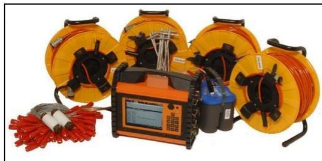
Fig. 1 - Electrical resistivity equipments
