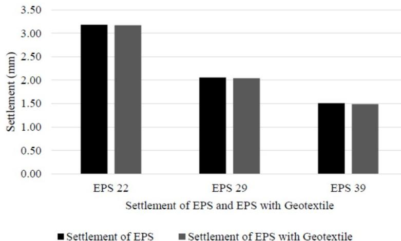
Fig. 11 - Settlement of EPS with and without geotextile
