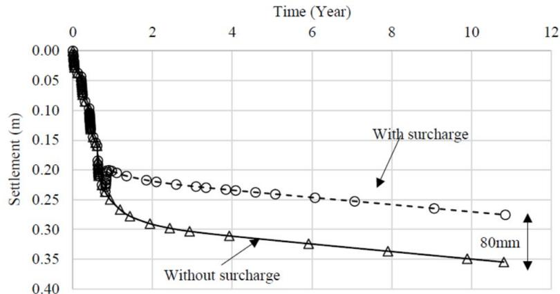
Fig. 5 - Settlement prediction of full stage construction of embankment with and without surcharge
