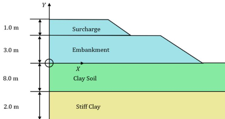
**Fig.1 - Geometry of the proposed model**
