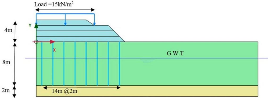
Fig. 2 - Conventional model with surcharge
