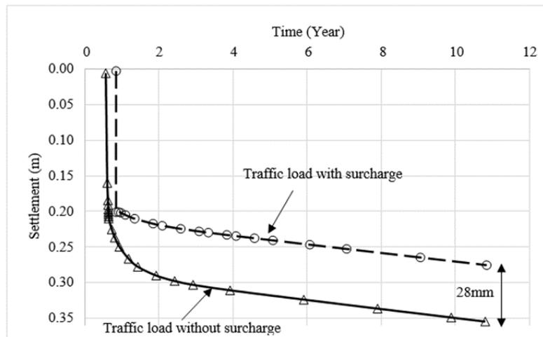
Fig. 6 - Settlement prediction considering the traffic load within 10 years
