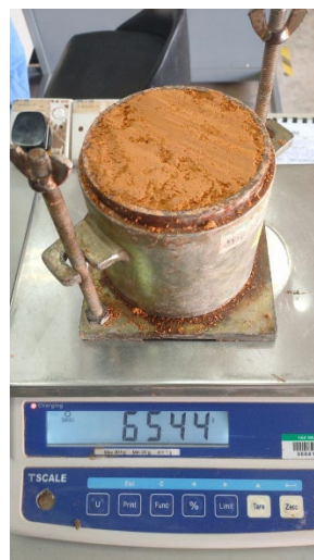
Fig. 1 - Soil sample after compaction
