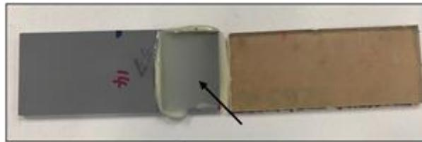
Fig. 3 - Adhesive failure (PVC & Acrylic)
