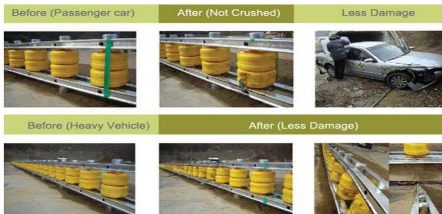
Fig. 10 - Crash test 2: car and truck accident at rolling barrier [20]
