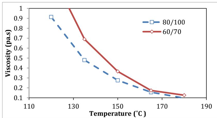
Fig. 5 - Viscosity versus temperature in asphalt binder grade 80/100 and 60/70
