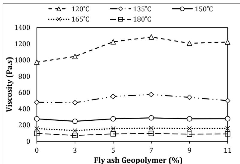
Fig. 6 - Relationship between viscosity and fly ash geopolymer content for asphalt binder grade 80/100
