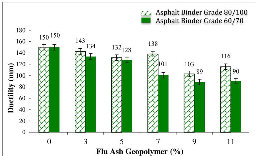
Fig. 4 - Relationship between fly ash geopolymer content and ductility for asphalt binder grade 80/100 and 60/70
