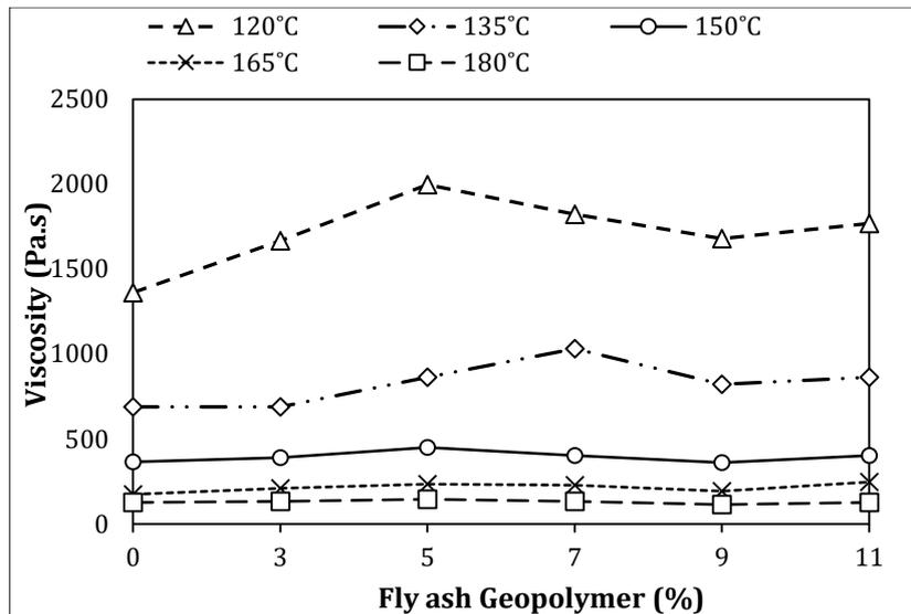
**Fig. 7 - Relationship between viscosity and fly ash geopolymer content for asphalt binder grade 60/70**
