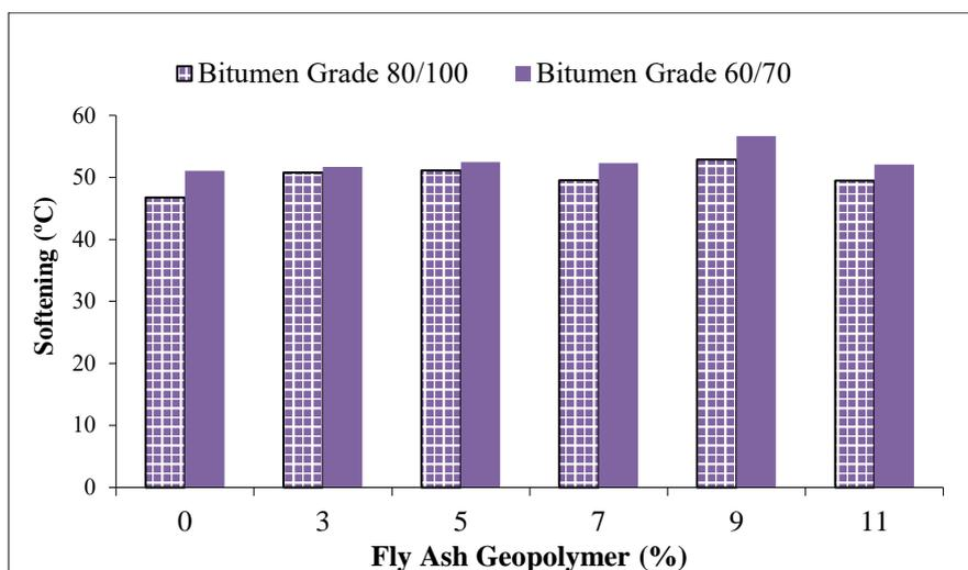
**Fig. 2 - Relationship between fly ash geopolymer content and softening point for asphalt binder grade 80/100 and 60/70**
