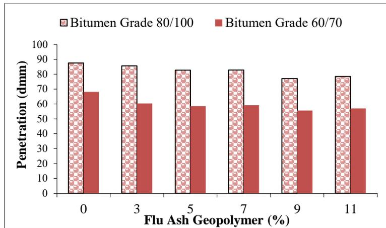
**Fig. 1 - Relationship between fly Ash geopolymer content and penetration for asphalt binder grade 80/100 and 60/70**
