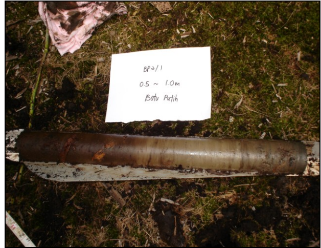
Fig. 3 Peat auger with sampled organic soil.
