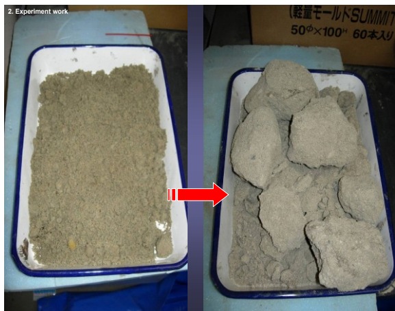
Fig. 8 Photograph of the untreated sample (left) and grouted sample (right).
