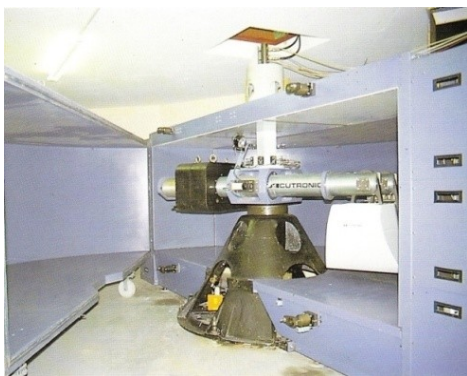
Fig.1 London Geotechnical Centrifuge facility: “Acutronic” 661 Geotechnical Centrifuge.
