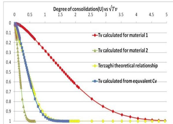
Fig. 6 Analytical Degree of Consolidation with Time.
