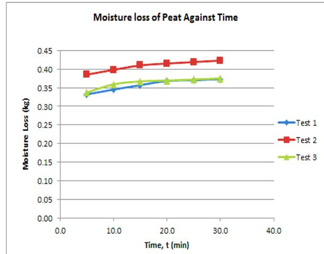
Fig. 3 Moisture loss of peat during sampling.
