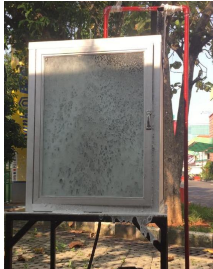
Fig. 9 - The outbreak of a sprinkler that sprays the extinguishing media
