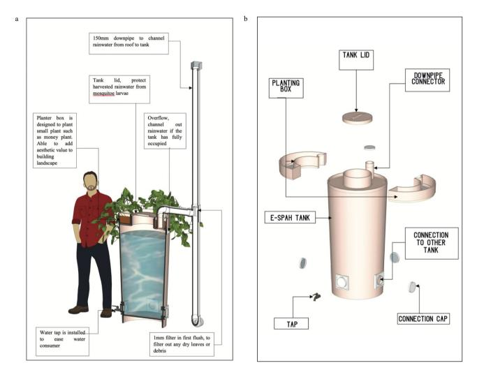
Fig. 3 - a) Sectional cut; b) axonometric projection
