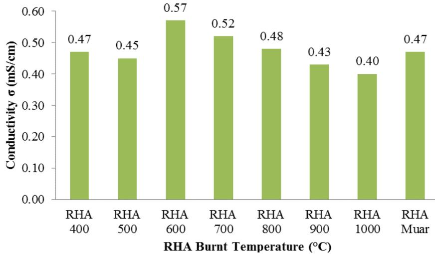
Fig. 4 - Pozzolanic reactivity with conductivity method
