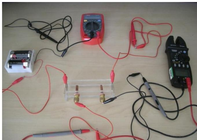
**Fig. 3 - Modified soil box resistivity test equipment**
