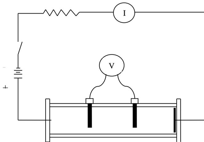
**Fig. 2 - Schematic diagram of modified soil box for resistivity measurement**
