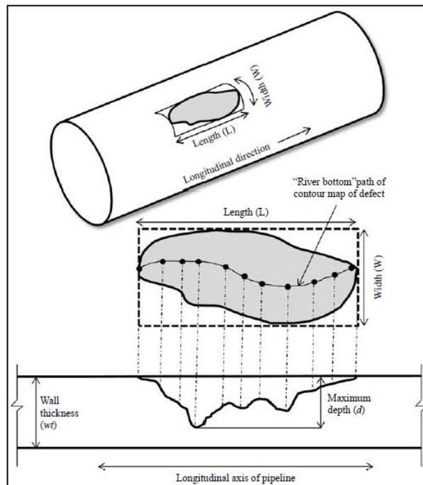
Fig. 3 - Volumetric loss due to corrosion in pipeline surface [15,16]
