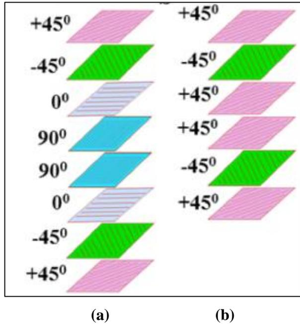
Fig. 7 - Schematic diagram of (a) symmetric quasi-isotropic laminate; (b) symmetric laminate [47]
