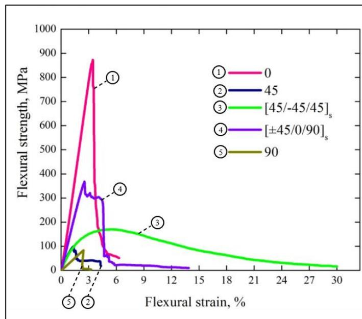
**Fig. 8 - The flexural strength versus flexural strain of CFRP [47]**
