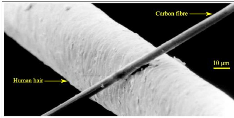
Fig. 4 - Comparison of carbon fiber with human hair [28]
