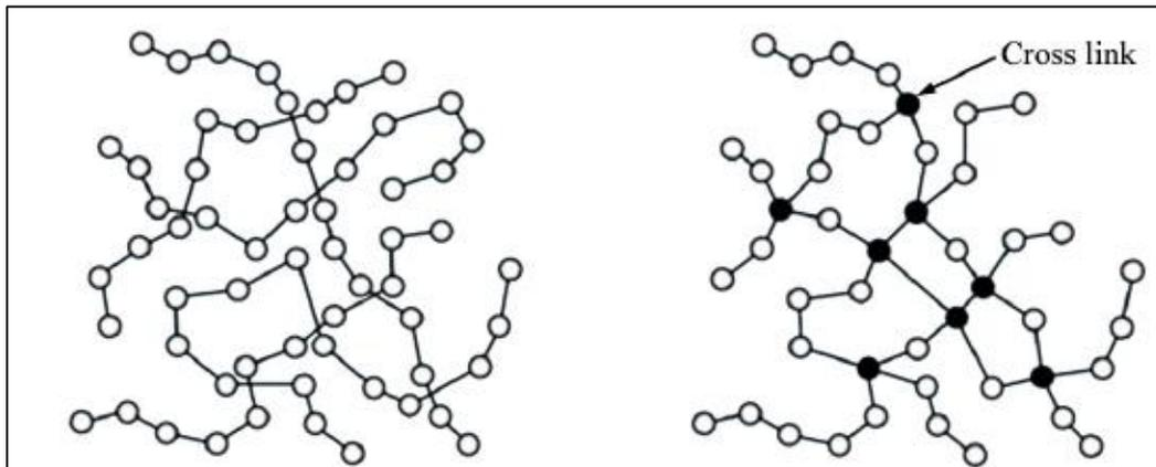
Fig. 5 - Molecular structures of (a) thermoplastic resins and; (b) thermosetting resins [39]
