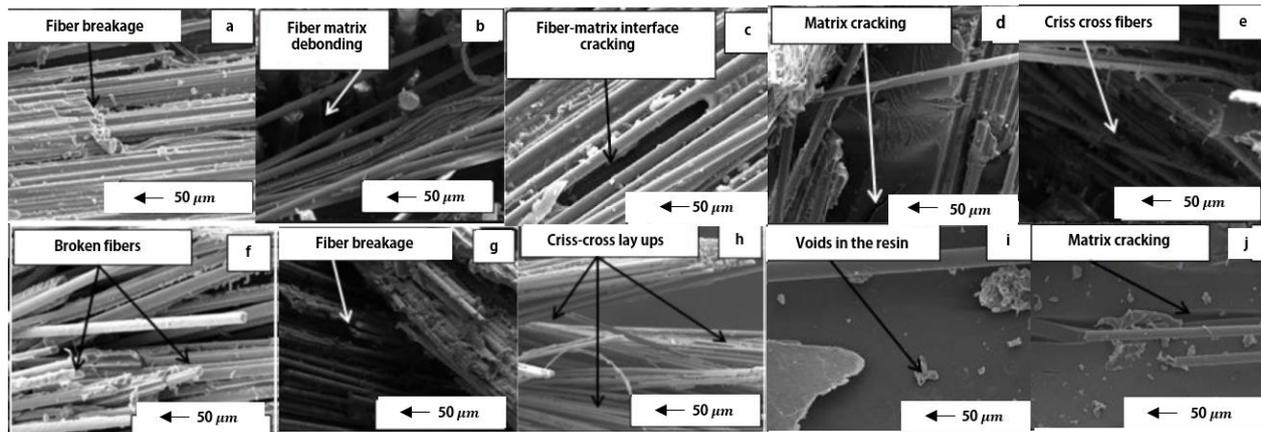
**Fig. 10 - SEM micrographs for different laminate orientations: 0° – a, b; 45° – c, d; (45°/-45°/45°) s – e, f; (±45°/0°/90°) s – g, h; 90° – i, j; CFRP – a, c, e, g, i; GFRP – b, d, f, h, j in bending [47]**
