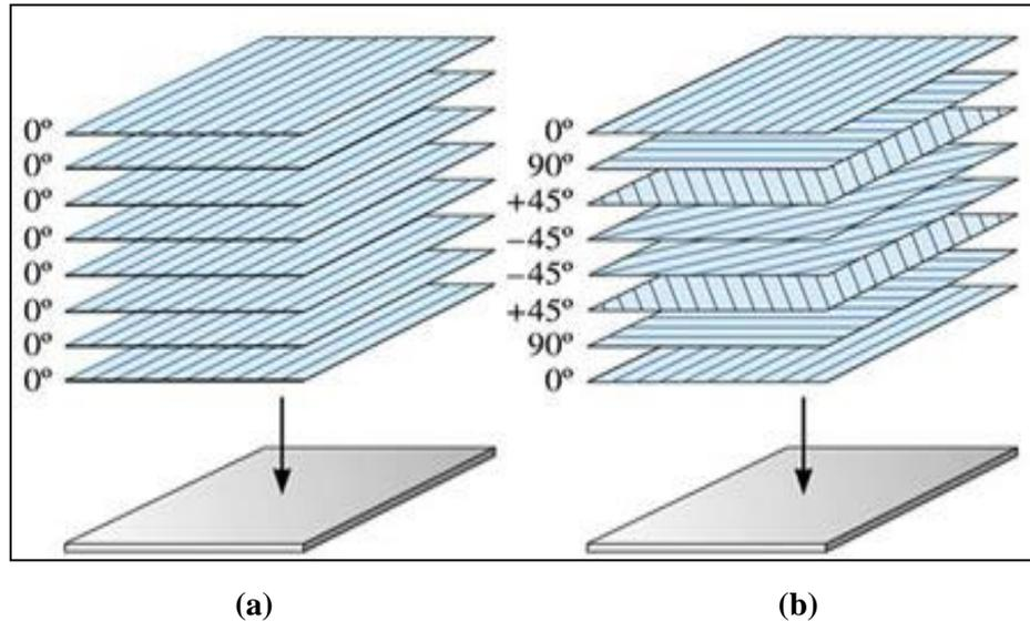
**Fig. 6 - (a) Unidirectional quasi-isotropic and; (b) cross-piled quasi-isotropic lamination [44]**
