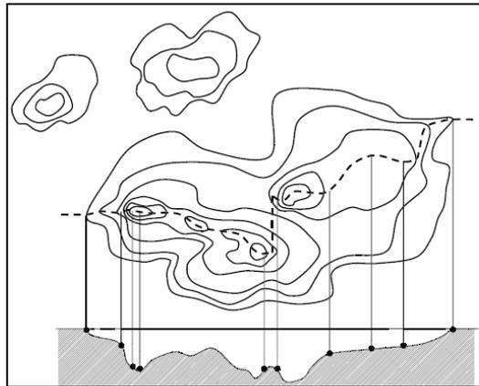
Fig. 2 - The irregular depth, width and length due to corrosion on a defected pipe [12]
