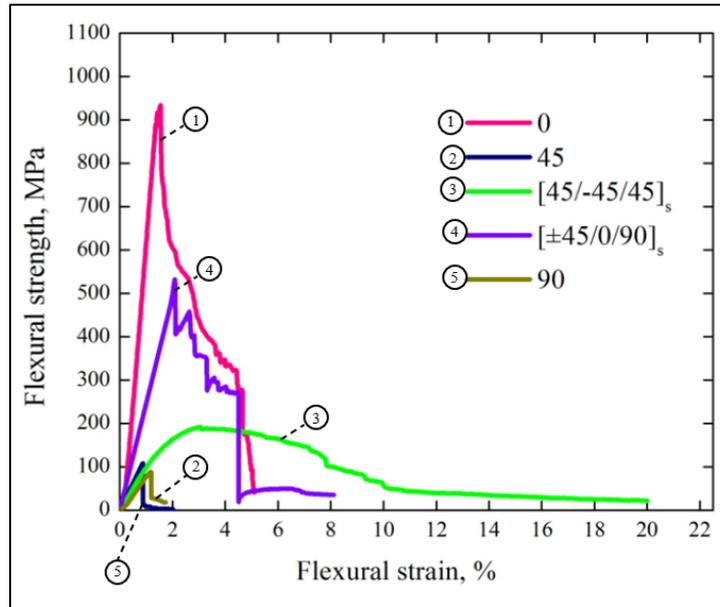
Fig. 9 - The flexural strength versus flexural strain of GFRP [47]
