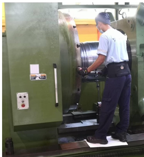
Fig. 8 - Photo of the machinist tightening the headstock jaws by using the manual torque multiplier and applying new methods
