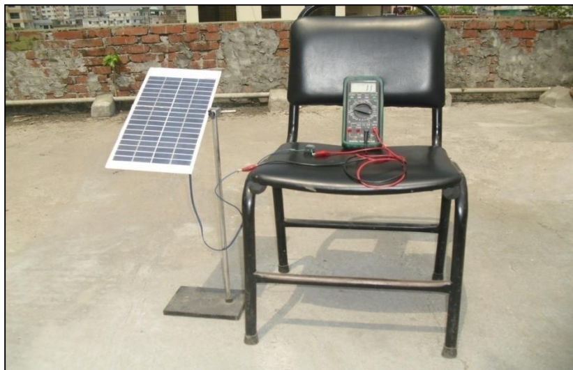
Fig. 6 - Photovoltaic system without solar concentrator
