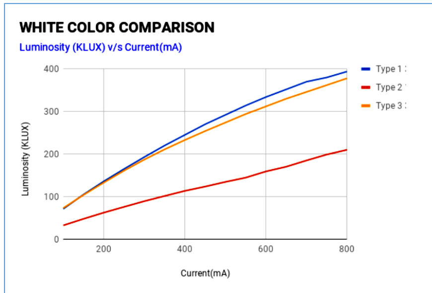
Fig. 10 - White colour illuminance comparison amongst three types of LED
