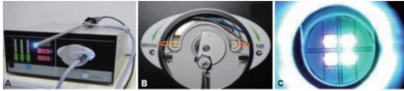
Fig. 1 - (a) NBI LED source PR650; (b) white LED light in the left side and blue/green (mix) LED light in the right side; (c) closed view of blue/green (mix) LED source}
