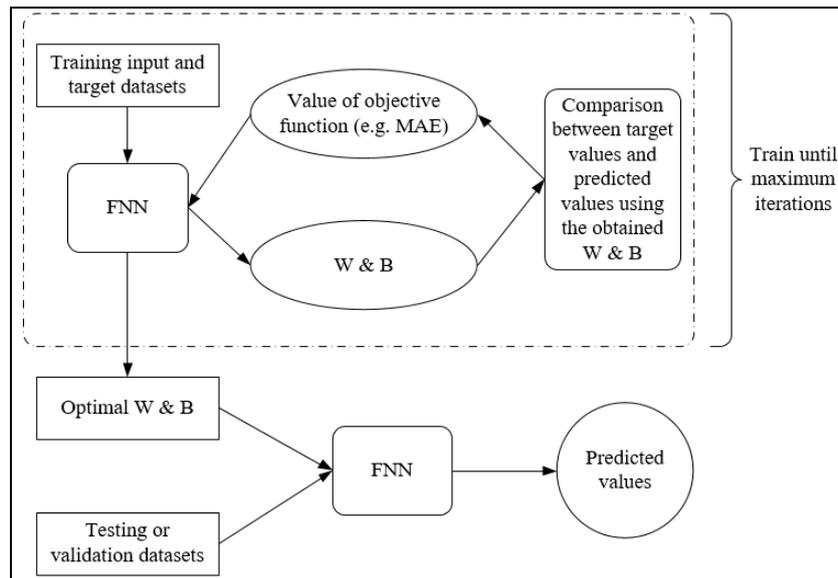
Fig. 7 - The optimization and prediction process of GWOFFNN, MVOFFNN, and MFOFFNN
