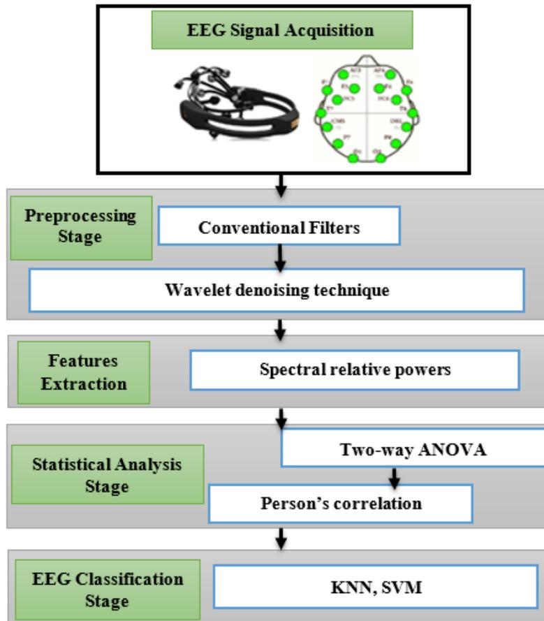
Fig. 1 - The block diagram of the proposed study
