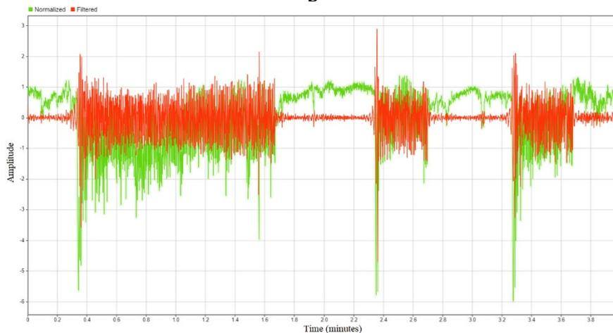
**Fig. 6 - Example of a pre-processed proximity signal normalized and filter using a bandpass filter of [1, 5], steepness=0.8**
