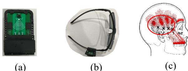
**Fig. 1 - Chewing detection system: (a) the proximity sensor into the 3D printed housing; (b) attachment of wearable sensor to the eyeglass; (c) temporalis muscle position**
