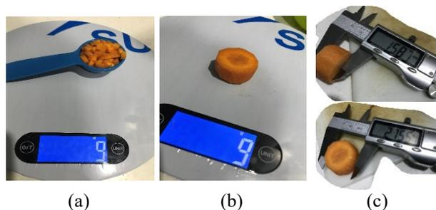
**Fig. 2 - Test food portion preparation and measurement: (a) one spoonful of test food being weighted, a cylindrical test food being; (b) weight; (c) measure**
