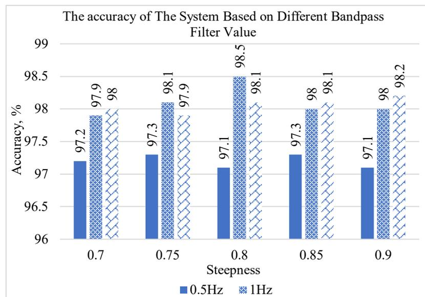
**Fig. 7 - The accuracy of the chewing detection system based on different bandpass filter values**
