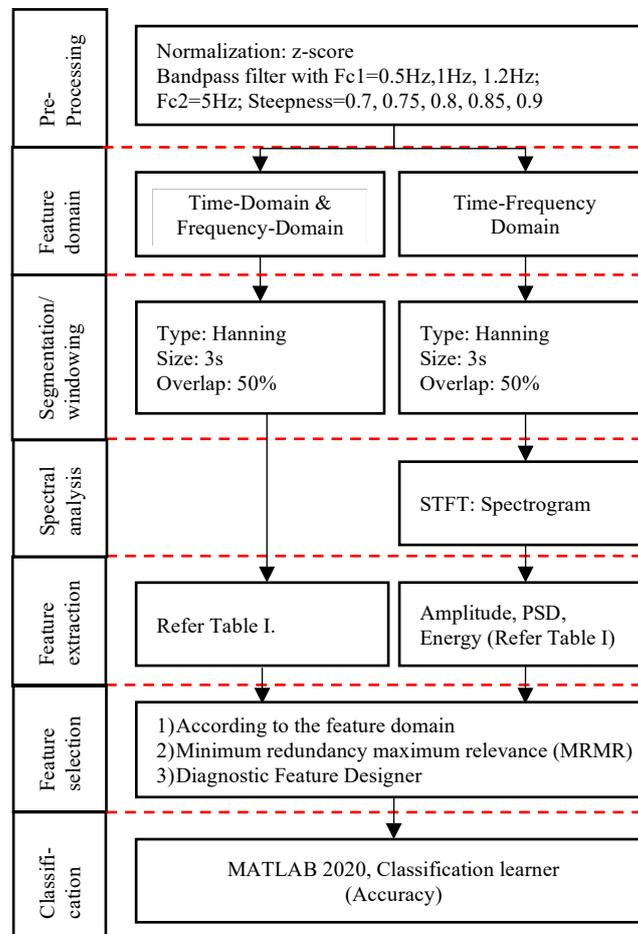
Fig. 5 - Signal processing pipeline
